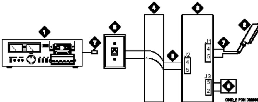
**Figure 11: Typical Non-registered Equipment Connections (Auxiliary Access)**
