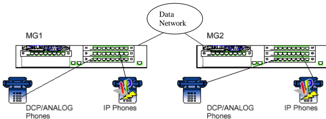
**Figure 8: MG1 with internal MGC, MG2 without internal MGC (DCP & Analog MM)**
