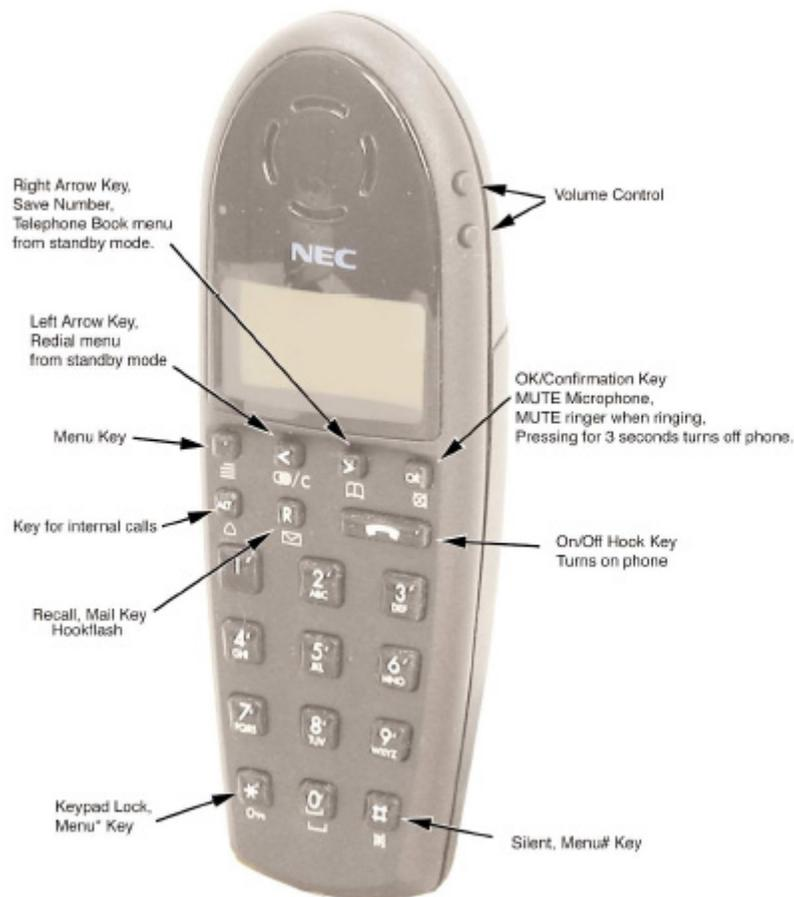
**Figure 13-33 DECT Wireless Telephone**
