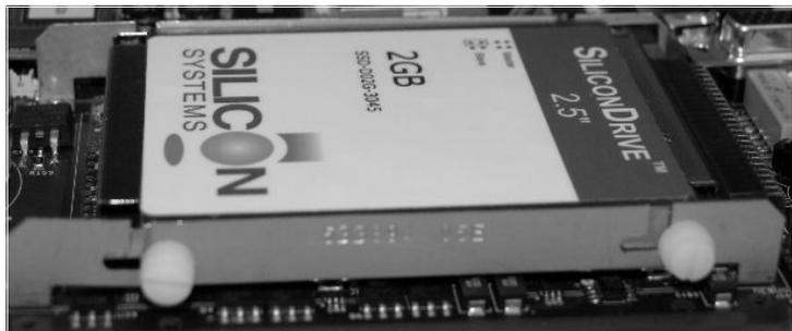
**Figure 6-52 Slide Drive Toward Connector**
