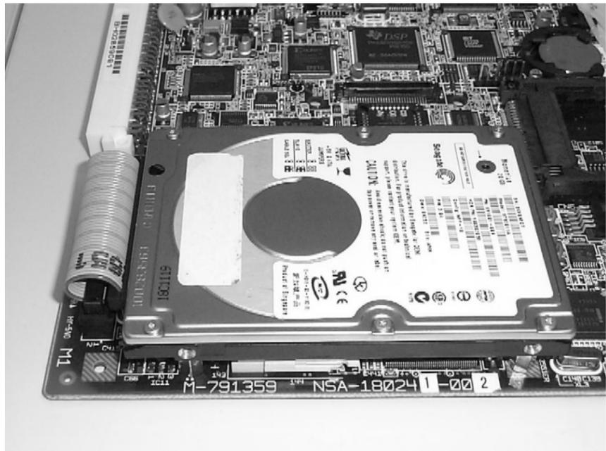
Figure 6-83 Placing the Hard Drive on the ETU
