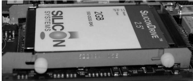
**Figure 6-55 Lift up and Remove Drive from ETU**
