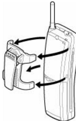
Figure 13-26 Removing the Belt Clip
