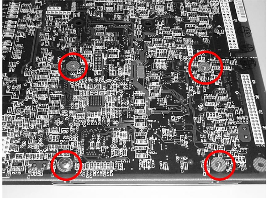
**Figure 6-84 Placing the Four Mounting Screws**
