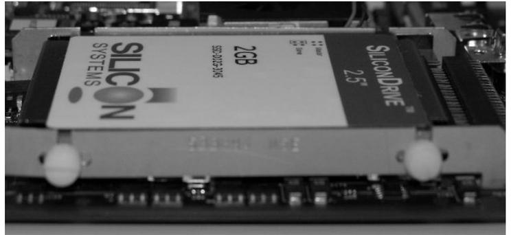
**Figure 6-53 Loosen the Four Screws**
