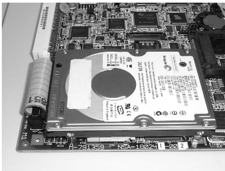
Figure 7 Placing the Hard Drive On the Card
