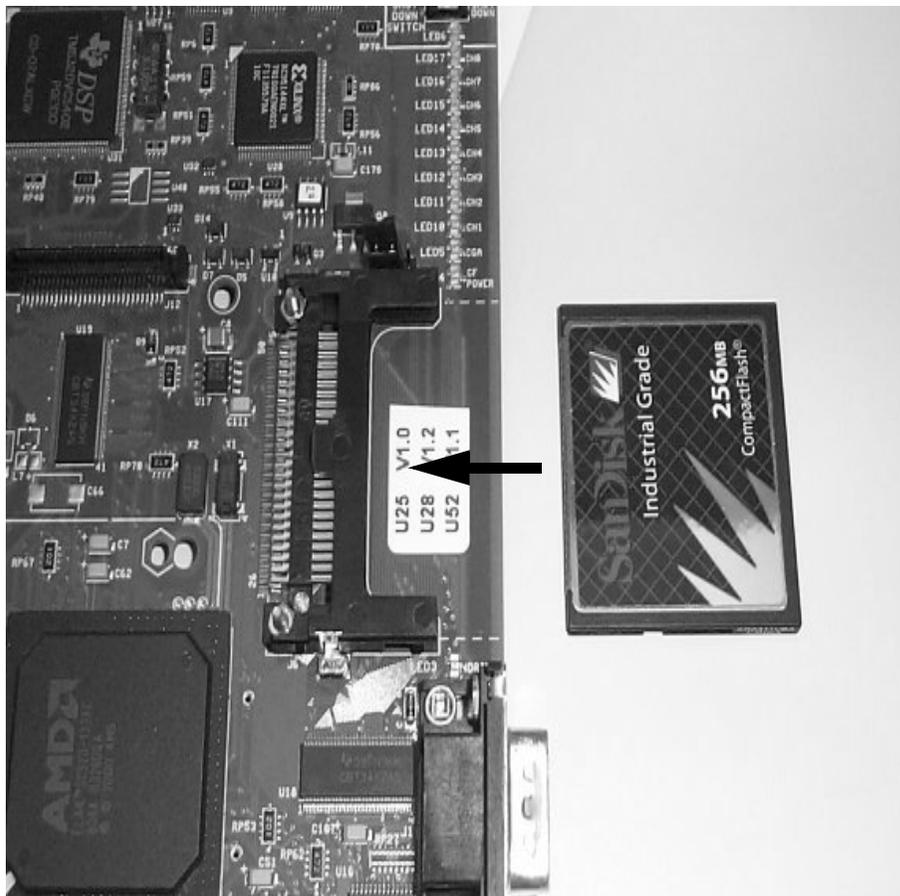
Figure 1 Installing the Flash Drive on the VMP( )-U40 ETU
