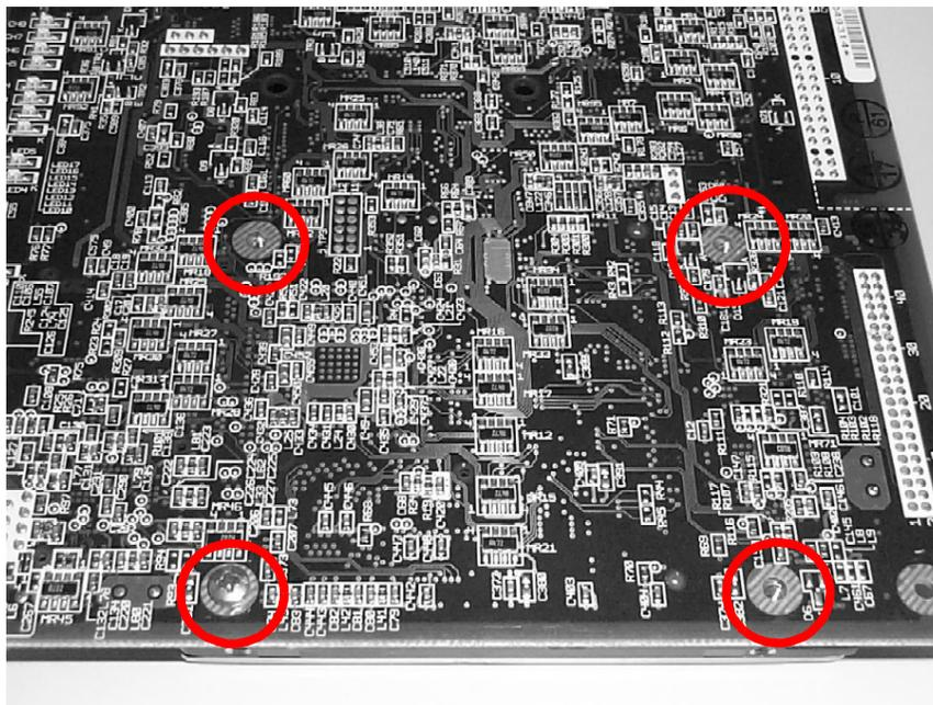
Figure 8 Placing the Four Mounting Screws
